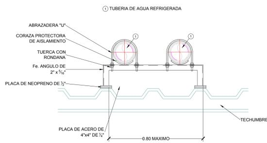
**DETALLE DE SOPORTE DE TUBERIAS ANCLADO AL PISO. (TUBERIAS BAJAS)**
